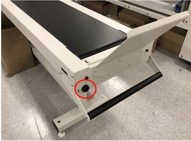
Heavies Divert Stacker Conveyor - Material Advance Button
