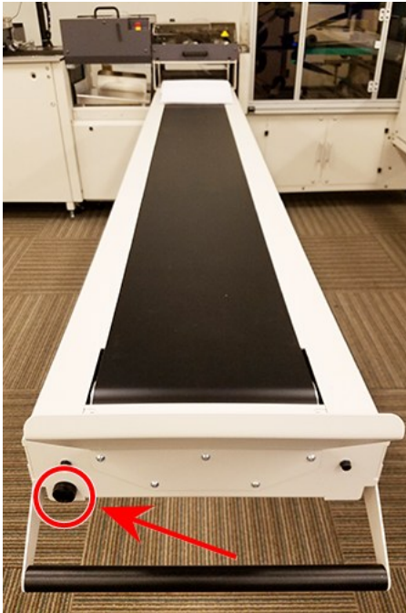
Shingling Conveyor - Material Advance Button
