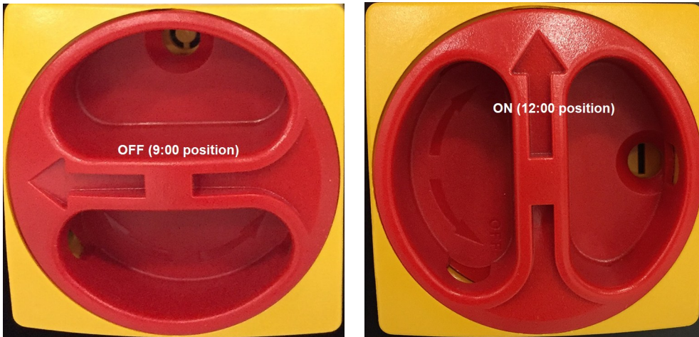
Main Power Switch - OFF position and ON position
